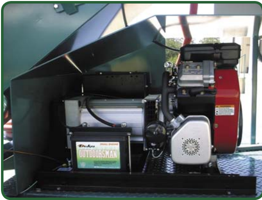
Propane Genset: Electric Start, Easy Operation and Maintenance, Provides Power to Conveyors and Burners
